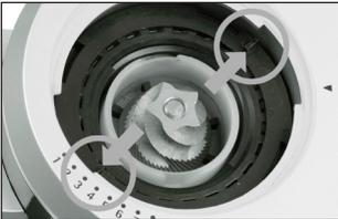
Check if the grinding block is in basic position. If necessary, turn the grinding block's ring **anticlockwise** as far as it will go until the two cones are positioned as in the picture.
